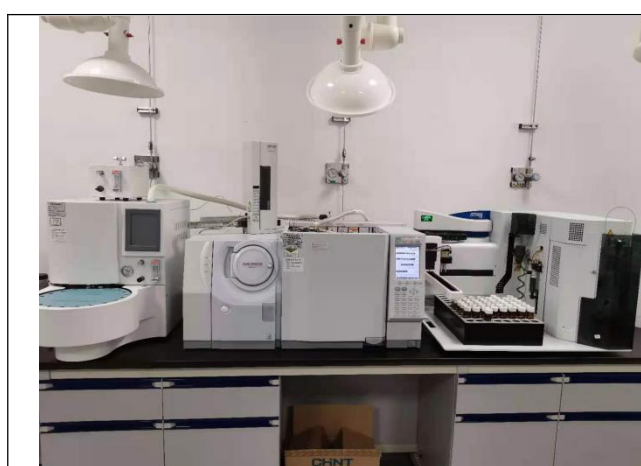
气相色谱质谱联用仪GCMS-QP2010SE
